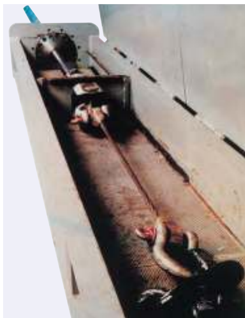
APPROVED TEST BENCH FOR UP TO 100 TONNES
