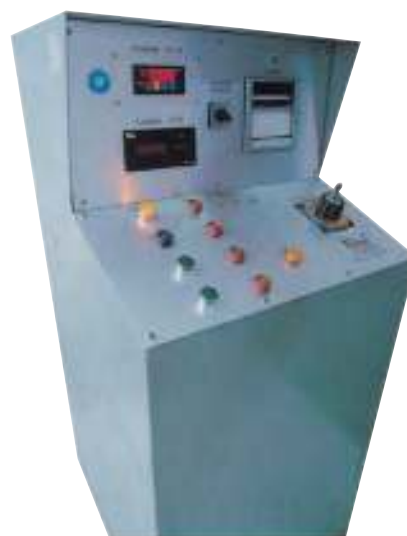
APPROVED TEST BENCH FOR UP TO 100 TONNES
