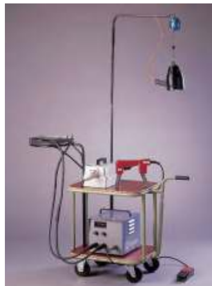
MOBILE CRACK DETECTOR FOR CHAINS AND ACCESSORIES
